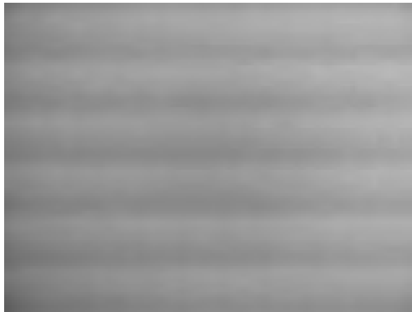
Figure 9: Flicker in image of white, uniform object illuminated by strong fluorescent light
